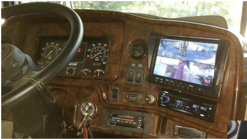
New monitor, showing metal mounting bracket attached to bottom of wooden frame and to bottom of monitor with small bot that fits threads in existing hole in bottom of monitor.
