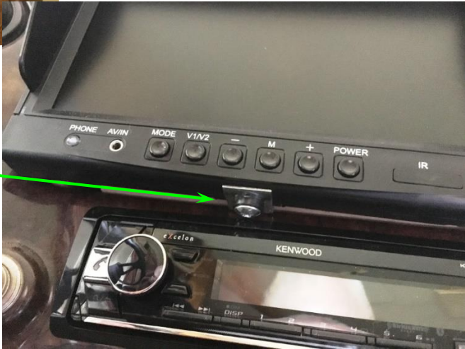
New monitor, showing metal mounting bracket attached to bottom of wooden frame and to bottom of monitor with small bot that fits threads in existing hole in bottom of monitor.
