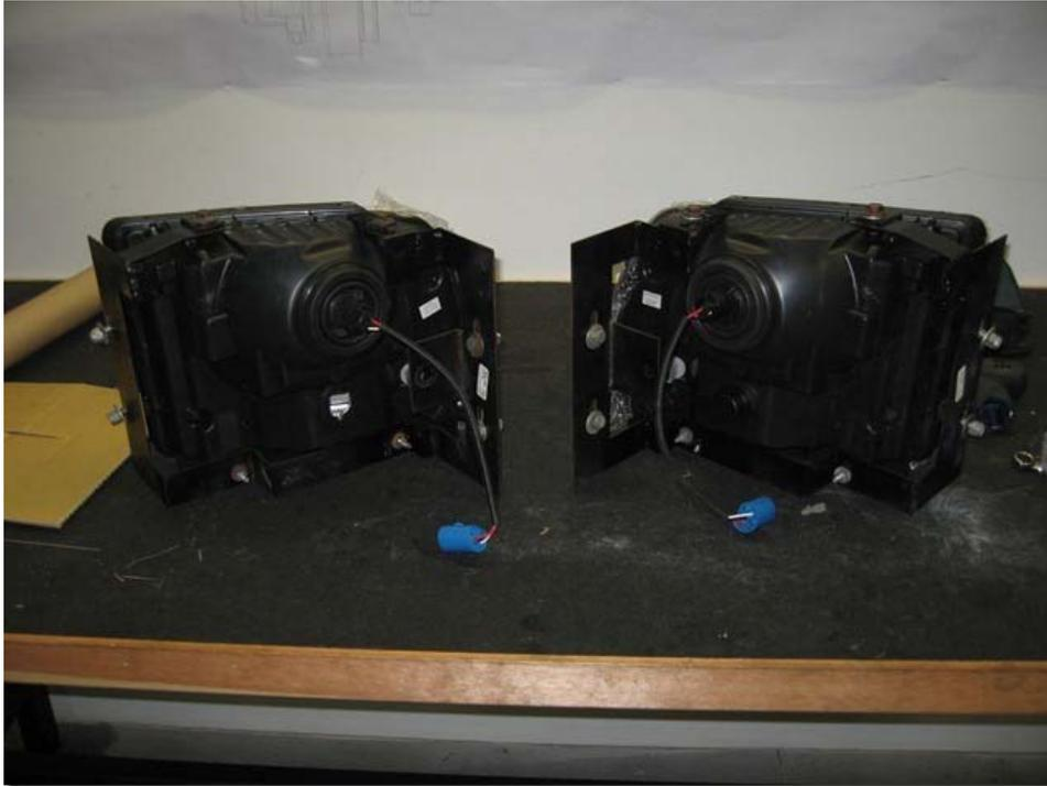
Here are the two new headlights bolted to the modified brackets. The two adapter harnesses convert the new bulb sockets to the old. They come with the kit.
