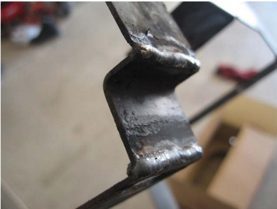
Bottom corner welded back on. Now the bottom will bolt flush.
