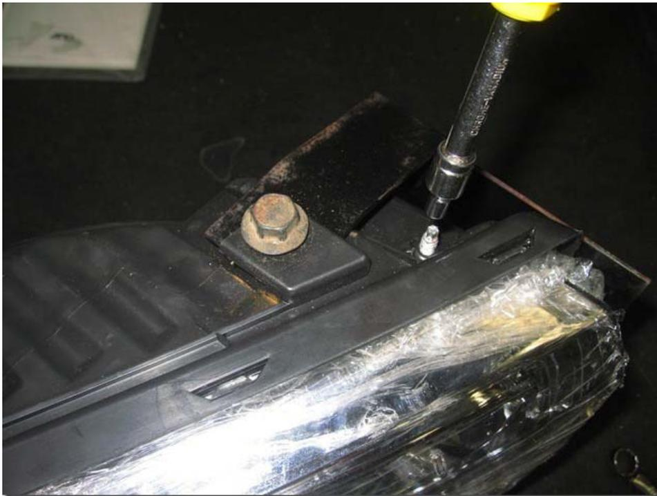
Here is the adjuster screw to align them, which you access in the front hood opening.
